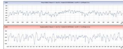
Roughness profile and primary profile
